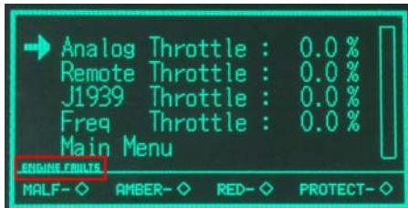
Figure 7. Fault Source for Engine
