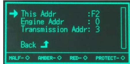
Figure 4: Address Setup Menu Example
